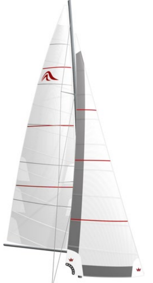
Conventional mainssail Material: Elvstrøm Blue Water Dacron white Layout: Cross cut
