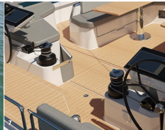
1 Two foldable helmsman's seats 2 Fwd Sun Pad Package 3 Cockpit table with teak top, electrically retractable to a lying surface 4 Throttle lever on instrument panel 5 Two GRP steering wheels, Y-spokes (black or white) 6 Second forestay with furling system 7 Two electrical LEWMAR 65 EST EVO sheet winches 8 Automatic fold-out bathing platform with remote control and bathing steps 9 Two additional electrical sliding hatches to both sides of companionway 10 Wetbar with BBQ, sink and fridge
